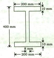
If the permissible stress is 150 N/mm<sup>2</sup>, the bending moment M will be nearly
