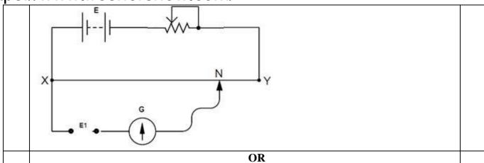
Following circuit was set up in a meter bridge experiment to determine the value X of an unknown resistance.
