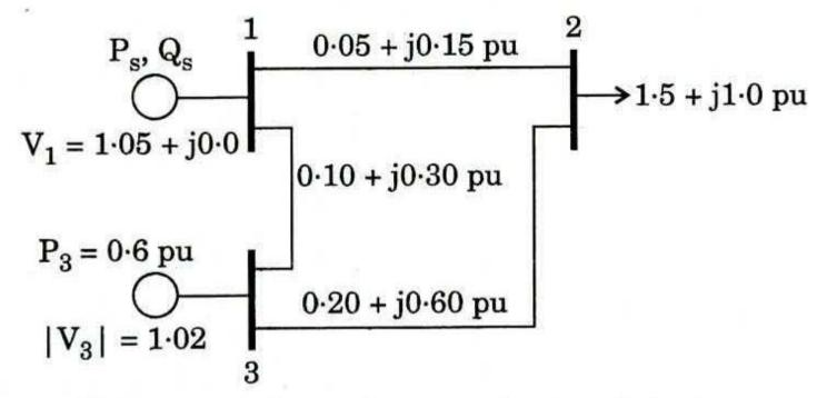
The per-unit bus voltages and power injections are also given in the figure.
